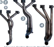
All Long Center Branch Manifolds have Y piece and gearbox clamps.
