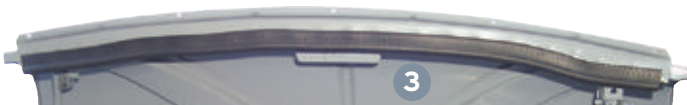
3. This seal fits on the front lip of the bonnet and does a great job on keeping the distributor and coil dry ..... JRC7898
