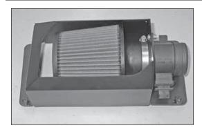
10. Install the K&N<sup>®</sup> air filter onto the mass air sensor inside the heat shield and secure with the provided hose clamp.
