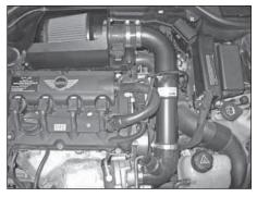
15. Install the K&N<sup>®</sup> intake tube into the silicone hoses on the turbo inlet and mass air sensor and then secure with the provided hose clamp.
