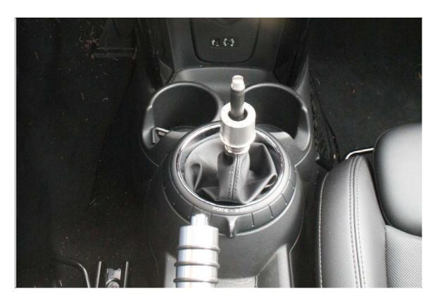
3. Place Knob Adapter over shifter. You'll notice a small collar on one end of the adapter, that collar will be facing DOWN, when you slide it over the shifter, it will click into the indented section (Seen below).
