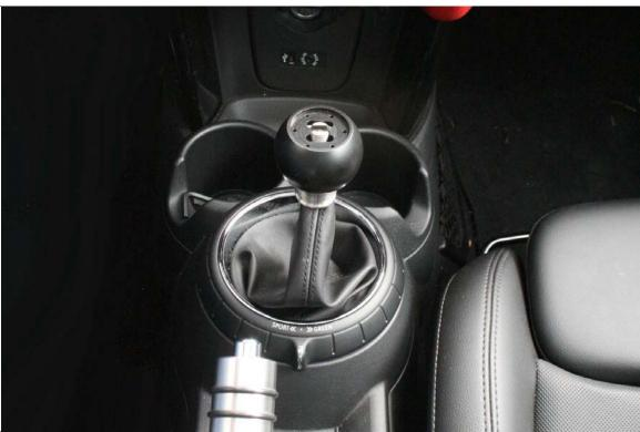
6. Make sure the holes in the knob, and core line up (You can grab the bottom of the core, and spin it)
