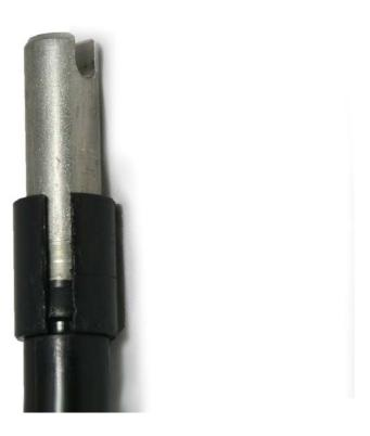
4. Slide Knob Core UP, but not off shifter, around knob core.
