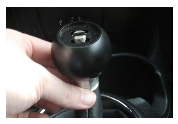
7. Place cap on your new knob, and install the 6 (2mm Hex) screws.
