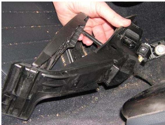
5. Get the Sprint Booster ready by plugging in the switch module – the little white connector goes into the white plug on the Sprint Booster. Much easier to do this in advance.
