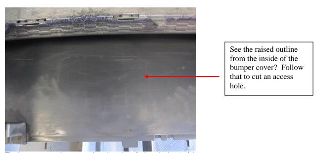
The bumper cover is now ready to be reinstalled on the back of the car
