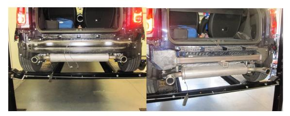
Remove the six 17mm bolts holding the steel bumper substructure to the car.
