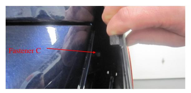
Picture 2 - Fastener C Under Rear Fender Flair
