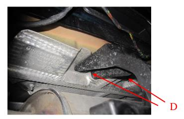
Picture 5 – Above Exhaust Fasteners D, 4 total
