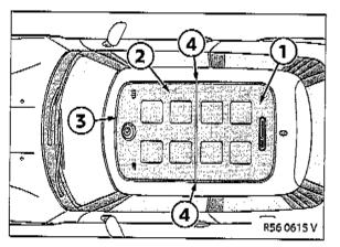
If necessary, when removing the black background film (1) and (2), wait **around 30-60 minutes** if the silver edging (3) starts to come away. The silver edging (3) must lie flush at the crossover points (4) with the sealing rubber of the glass roof.
