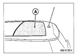
Place the transfer paper bearing film segments  $\bf A$  on the underside on the rear area of the glass roof. Align the transfer paper with the glass roof frame as you do so.
