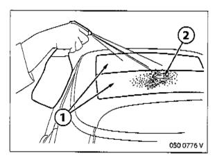
Clean the glass roof with a cleaning cloth and suitable cleaning agents. The glass roof must be completely dry, clean and free from wax or grease.
