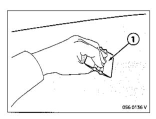
Repeatedly spray the sections with installation solution. This makes spreading easier and avoids damage to the film or the glass roof.
