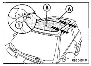
In order to avoid damaging the surface of the roof, do not run the blade beyond the glass roof area.
