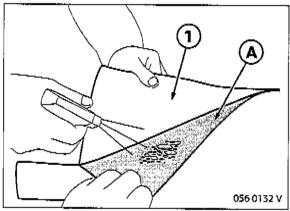
The film sections for gluing are supplied on transfer paper **A**. The adhesive side of the sections is covered with a printed protective film (1).
