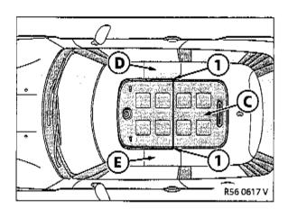
Place the transfer paper with film section C between the two templates D and E and align it with the corner contour (1) of templates D and E, press down firmly and run the blade over it.
