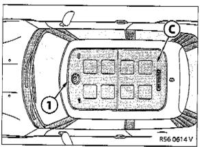
Lay the two film sections **C** along the contour (1) of the glass roof, align them and run the blade over them. Spray the application tape with installation solution and carefully remove it after **around 5 mins**.
