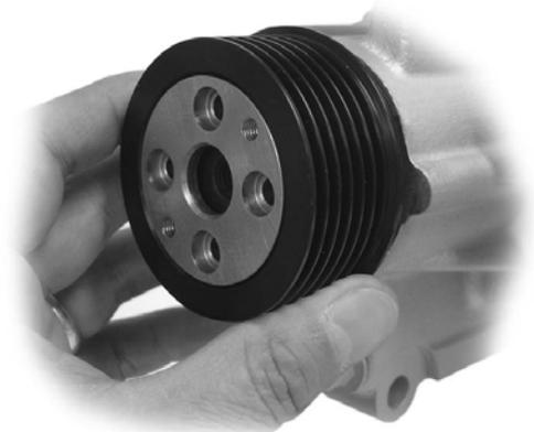
3. Align the front and rear collars and insert the bolts. Start the bolts by hand to make sure they are not cross threaded.
